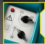
The dashboard, locate on the hood, is very si and includes: vacuum cut-off device side brush raising\lov key switch.
