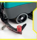
AUTOMATIC SQUEGEE UNCOUPLING when accidentally impacted avoids damage to the machine or to the environment.
