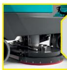
THE SCRUB DECK is equipped with a self-adjusting splash-skirt which, besides preventing the dirt water to splash during the cleaning session, allows for water-leaking prevention.
