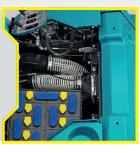
Strong hydraulic drive system, variable speed controlled up to 9 Km/h, by means of two pedals (fwd & rev)
