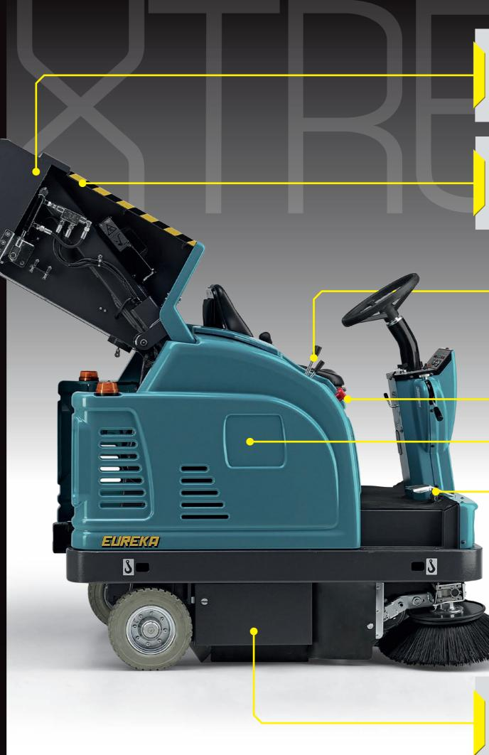
The multi-level-dump hopper, equipped with hydraulic flap, is located in the rear of the machine. It can be hydraulically raised up to 1.360 mm from the floor, and has a volume capacity of 150 litres.
