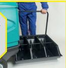
The floating, self-levelling main brush can be quickly adjusted or replaced without tools, and the retractable, anti-shock side brushes ensure maximum cleaning efficiency on rough or uneven floors.
