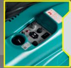
All controls are simple to use and ergonomically designed for easy operation. One single pedal controls forward and reverse speed; the levers to lower or raise the main and side brushes are located on the dashboard, as well as the filter-shaker control and the vacuum cut-off device, which can be engaged when sweeping on wet areas.
